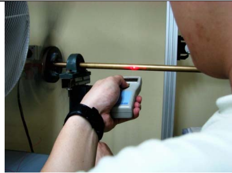
b. Student measuring the wind turbine airfoil speed.
